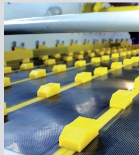
Pro-CLIN® slotted screen panel system for screening machines
