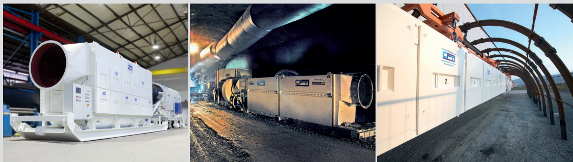
CFT dry-type dedusting units for heading processes in mining and tunnelling
